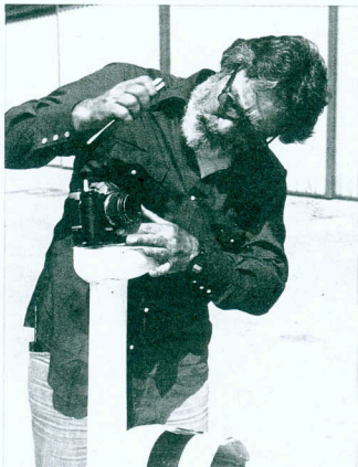
The author loads his wing tip camera prior to installing the streamlined fairing over it.
