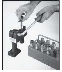
Since the Champion Model 2500A gapsetting tool adjusts two electrodes simultaneously, it is particularly useful for highvolume gap-setting requirements. This tool easily adjusts four-electrode N Type and two-electrode E Type aviation spark plugs.
