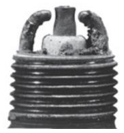
The REM37BY Extended Core Nose spark plug does not prevent the accumulation of lead deposits, but its design makes it capable of firing with severe lead deposit buildup.
