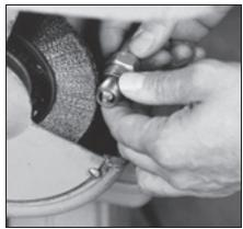
Cleaning threads with a rotary brush.
