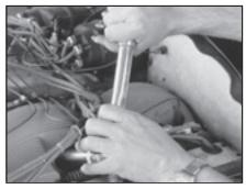
Tightening spark plugs with torque handle.
