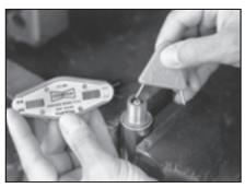
Setting gap on fine-wire spark plug.
