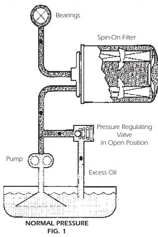
the point that many mechanics that are not familiar with lube systems fail to realize. Just remember any blockage in the system can also send the pressure beyond what the filter can stand which is rated at 400 psi. Burst.
