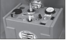
Cleaning firing end with model CT-475AV Cleaner/Tester. The CT-475AV requires P/N 91893 Abrasive Compound, 15-ounce size.
